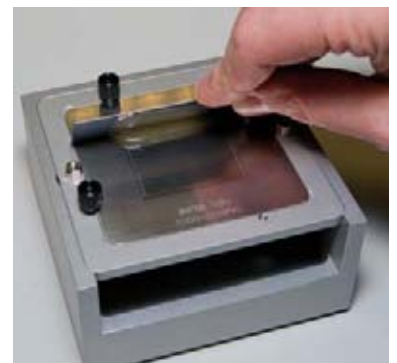
Flux deposition in the dipping stencil
