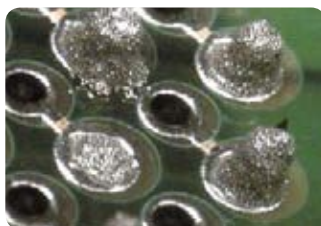
BGA – paste print: insufficient solder
