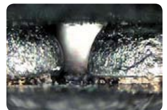
PBGA – scaling: insufficient heat
