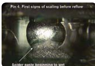
PBGA – scaling: insufficient heat
