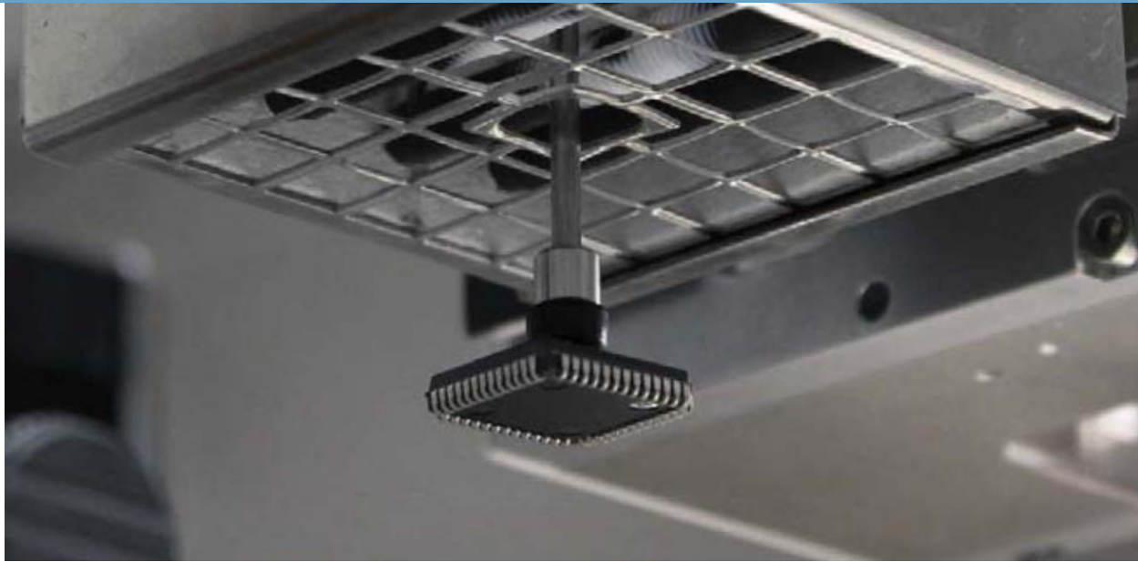
Desoldered PLCC component
