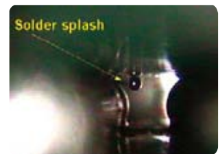
BGA: via hole solder splash
