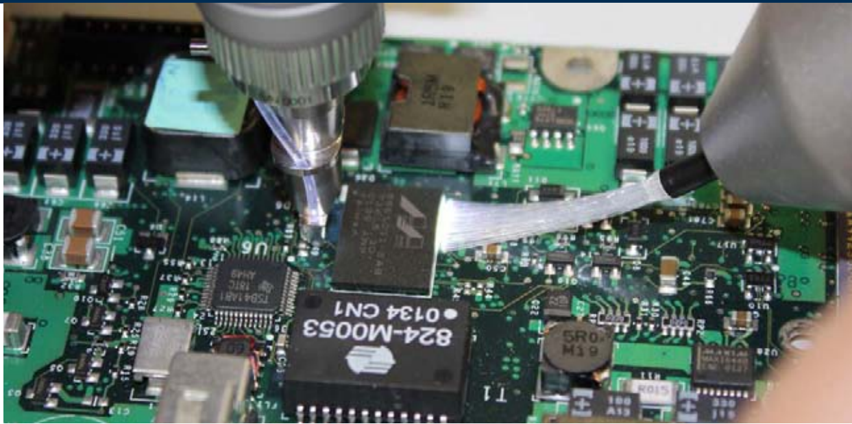
Inspection of a CSP
