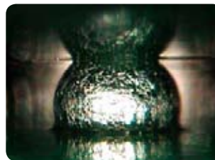
PBGA – scaling: insufficient heat
