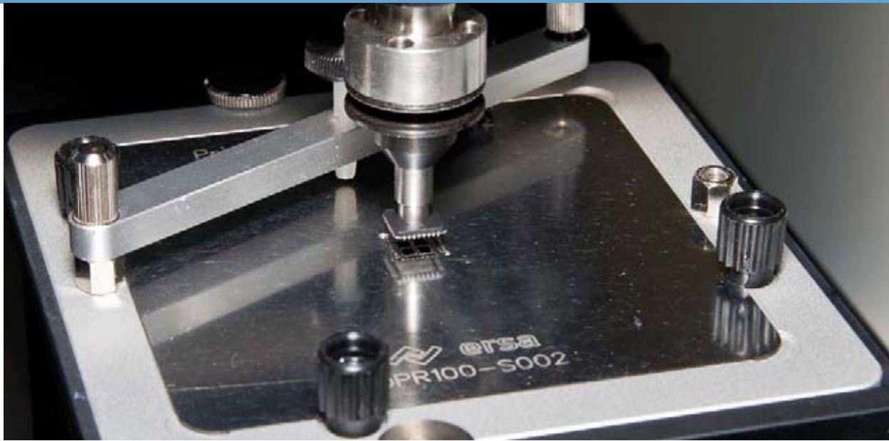
Removal of the component from the printing stencil
