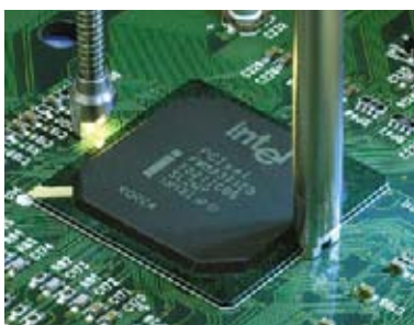
ERSASCOPE 1 fixed optics for BGAs;
