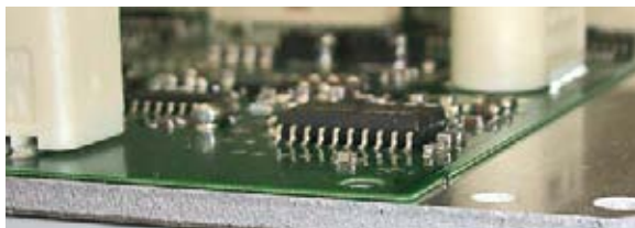
SOIC & Plastic SMT on Aluminium Carrier
