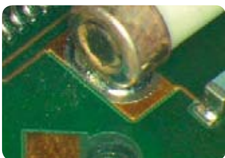
Lead free assembly: non-wetting
