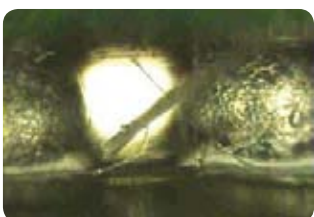
Flux residue under BGA
