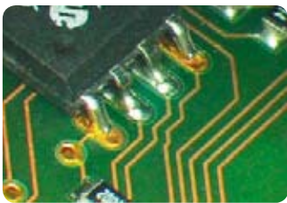
Lead free assembly: non-wetting
