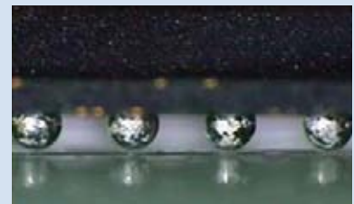
Real-time rework process visualization of BGA during reflow
