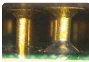
PGA: insufficient hole fill
