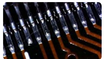
QFP solder joints – taken with the Ersca MOBILE SCOPE Macro Zoom Lens
