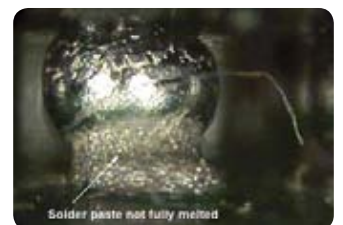
PBGA – scaling: insufficient heat
