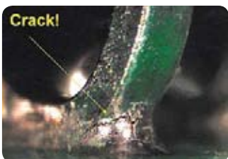
Lead free PLCC: micro crack
