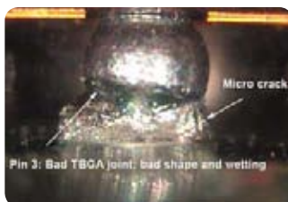
TBGA: disrupted joint & micro crack
