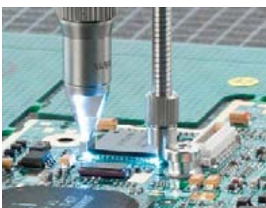
ERSASCOPE 2 Exchangeable optics for CSPs
