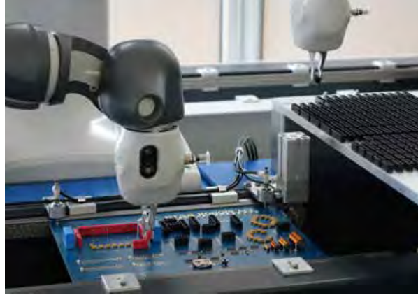
Individually programmable, simultaneously operating arms
