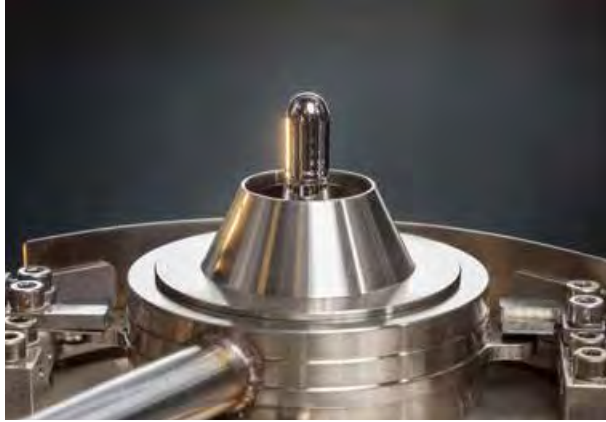
Single nozzles – used on single or dual pot, subject to the solder module
