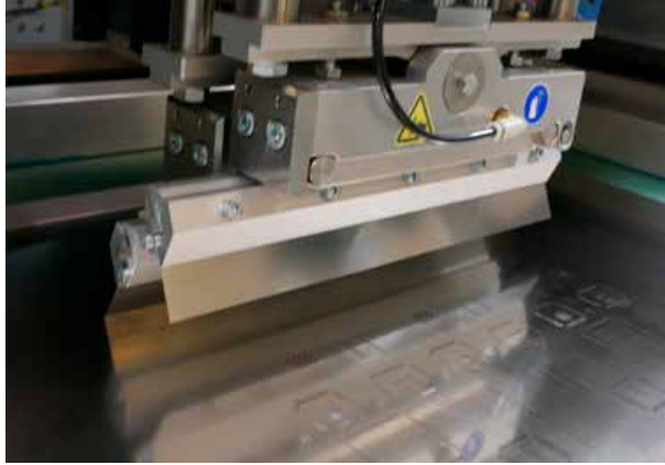
Printerhead and squeegee with paste height control
