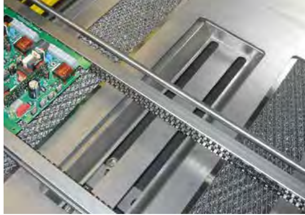
Precise flux deposition with precision spray fluxer
