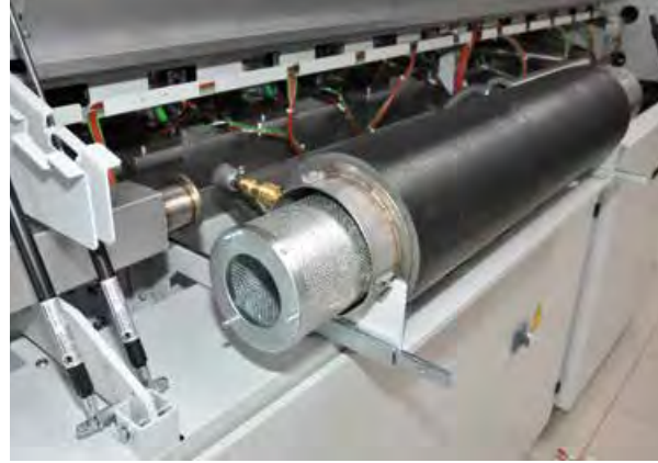
Condensation management with cleaning granulate
