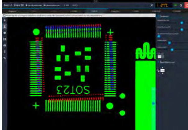
Rework made easy with computer assisted component placement
