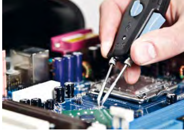
Precise desoldering of SMDs with the Ersa CHIP TOOL VARIO
