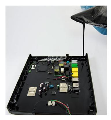
Resins are widely used for potting and encapsulation in the electronics and electrical industries, and are generally found in three major categories, depending on their chemical types: epoxy, urethane and silicone. Electrolube develops, manufactures and supports a wide variety of resin products within these categories.
