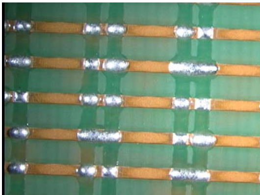
Figure 2 . Wetting test cross-print post reflow
