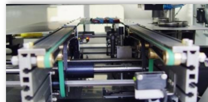
▲ Three-Step Independent Conveyor (Cut-view of Entry Conveyor)
