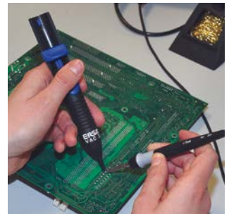
Sucking up the old, molten solder remnants with a mechanical solder sucker (desoldering pump)
