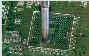
2. Remove residual solder from the pads of the board
