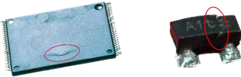
Illustration 1: Visible MSDs Damaged During Reflow Solder
