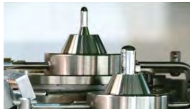
Dual solder pots with soldering nozzles in different shapes
