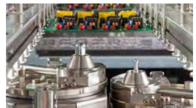
Innovative y/z-variable dual solder pot system
