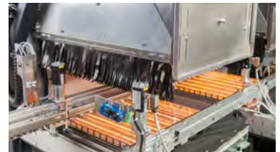
Speed regulated, full area convection for individual preheating performance
