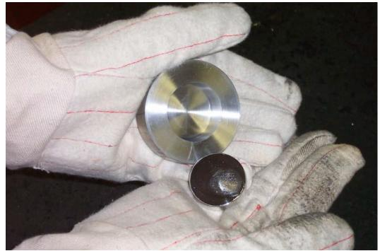
After the sample cools, turn the mold over and the sample should fall out.
