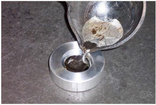
Continuously pour your sample into the mold filling it up ¾ full. Let stand until sample completely solidifies and cools.
