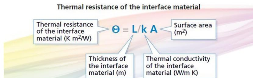
there are no pockets of heat created throughout the unit. In order to achieve this, the resin will have to have the correct combination of thermal conductivity and viscosity; typically, as the thermal conductivity increases, the viscosity also increases. Electrolube offer specialist resins to help reduce viscosity for ease of application, whilst maintaining a high level of thermal conductivity for efficient heat dissipation.
