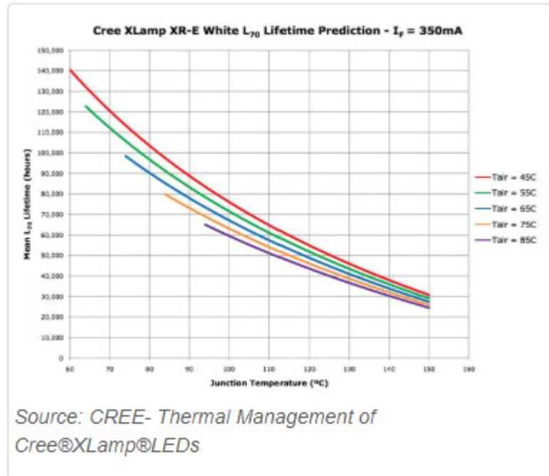
Ensuring efficient thermal management is employed will therefore provide consistent quality, appearance and lifetime of LED arrays and in turn, opens up the opportunity for further applications for this ever evolving industry.
