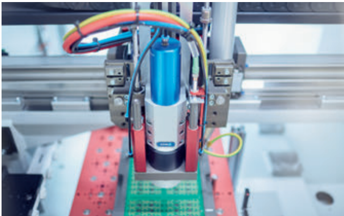
The basic configuration consists of a milling bit module. As optional expansion of the base system, the milling bit module is available with a vision system, as well as a scanner.
