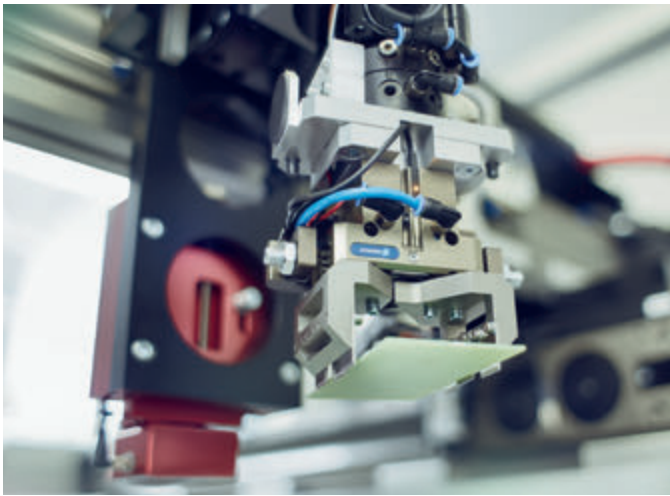
Simple and light-weight grippers for PCB handling are cost effective and guarantee the shortest cycle times with the most flexibility.
