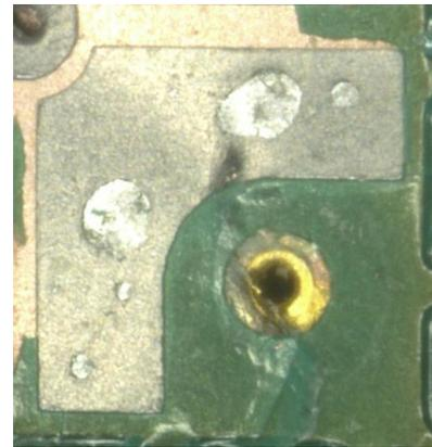
**Figure 13:** Corrosion path at the encroached via
