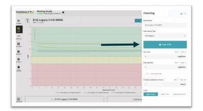
The Assign Profile form will automatically import your board and test information as well as calculate the six-sigma upper and lower specification limits for each channel.
