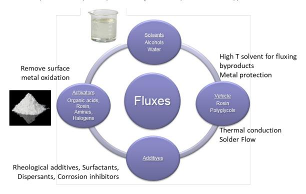
Flux compositions are highly complex engineered materials. Whether soldering with a no-clean, washable no-clean or water-soluble flux, the propensity of the remaining residues to cause electrochemical failures needs to be quantified. SIR is the best test method for determining activity of these residues.
