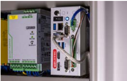
INDUSTRY 4.0 on board: The Gateway Kurtz Ersa GATE ensures safe, standardised connections between Ersa systems and the outside world.
