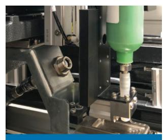
Ensures paste is at optimal temperature for best printing results
