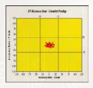
XY dot placement accuracy +/-35 microns @ 3 sigma at full system speed 1.5g of peak acceleration
