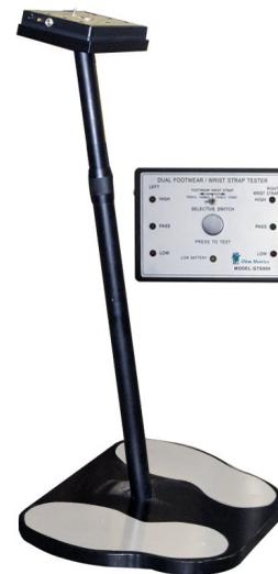
Deluxe three-state touch tester designed for fast and accurate testing of ESD ground devices. A unique dual test circuit eliminates the need for separate wrist-strap and foot grounder testers which saves money and space. Both feet can be tested at the same time.
