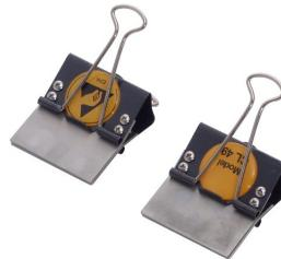
Designed to evaluate ESD garments. A wide stainless steel surface ensure excellent contact during testing.
