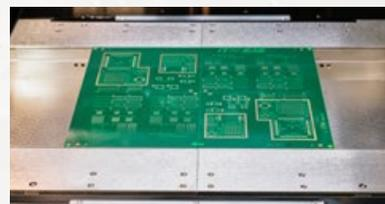
The EdgeLoc system uses a side snugging technique that removes the need for top clamps which interfere with the PCB to stencil contact.
