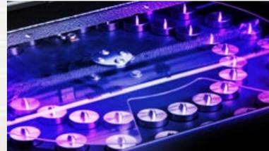
Automatic Pin Placement is MPM's patented tooling solution that uses the vision gantry to precisely place and remove tooling pins.
