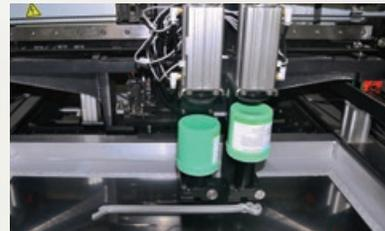
Dispense for standard cartridges or choose the new patent-pending jar dispenser. Paste is released in precise, measured amounts across the stencil in a
