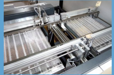
Both short-wave IR emitters can optionally be upgraded with top-side convection heaters
