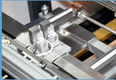
High-precision spray fluxer with integrated spray jet control
