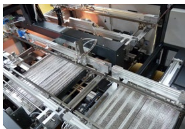
In- and offline selective soldering system in a U-shape arrangement for modern manufacturing layouts
