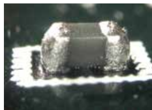
0402: bulbous solder joint
