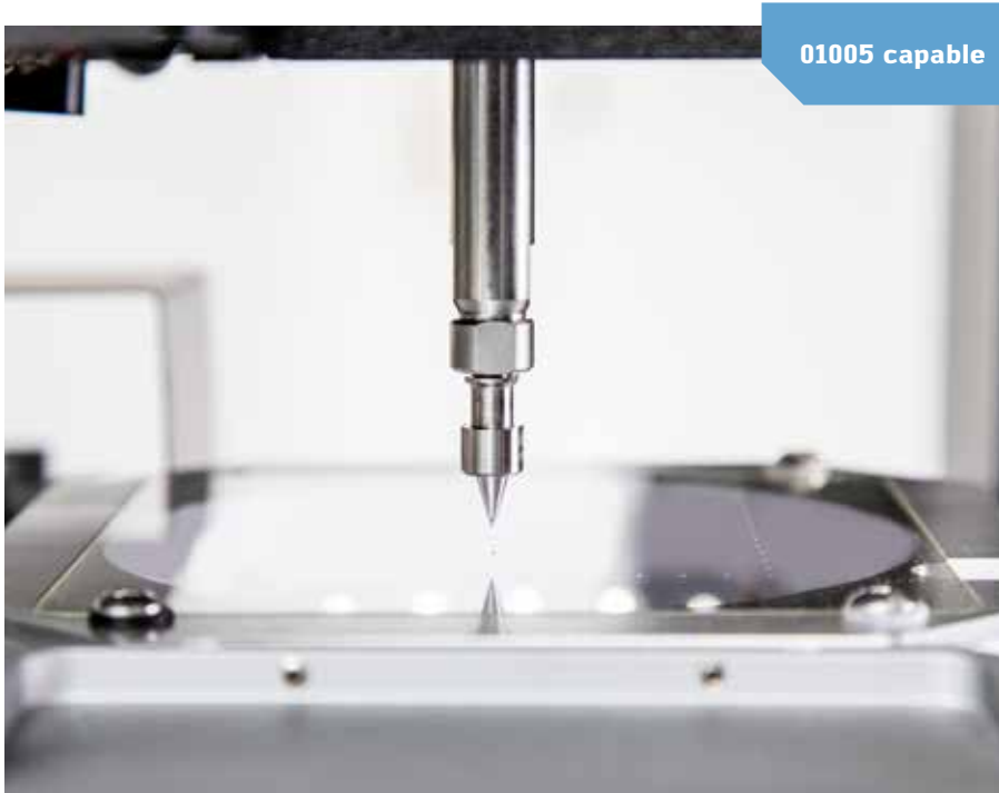
Automatic pick-up of a 01005 chip
