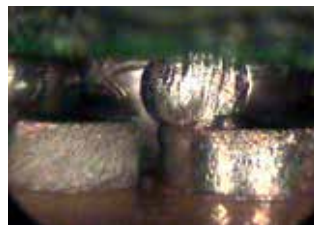
BGA – piggy back: bad alignment
