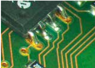
Lead-free assembly: non-wetting
