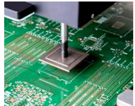
Handling of a metallic BGA
