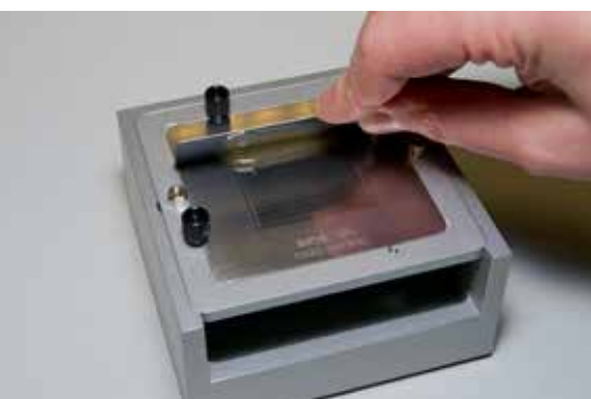
Flux deposition in the dip stencil
