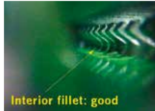
PLCC – interior fillet inspection
