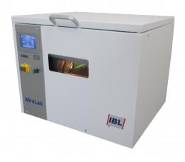
The MINILAB vapor phase machine is characterized by it's compact design and the easy handling. Her element, the mini series production, she masters bravely and guaranteed at the same time highest solder quality. Especially she was designed for development and prototype production as well as for soldering BGAs and LGAs. Due to its small footprint, it's quickly ready for use.
