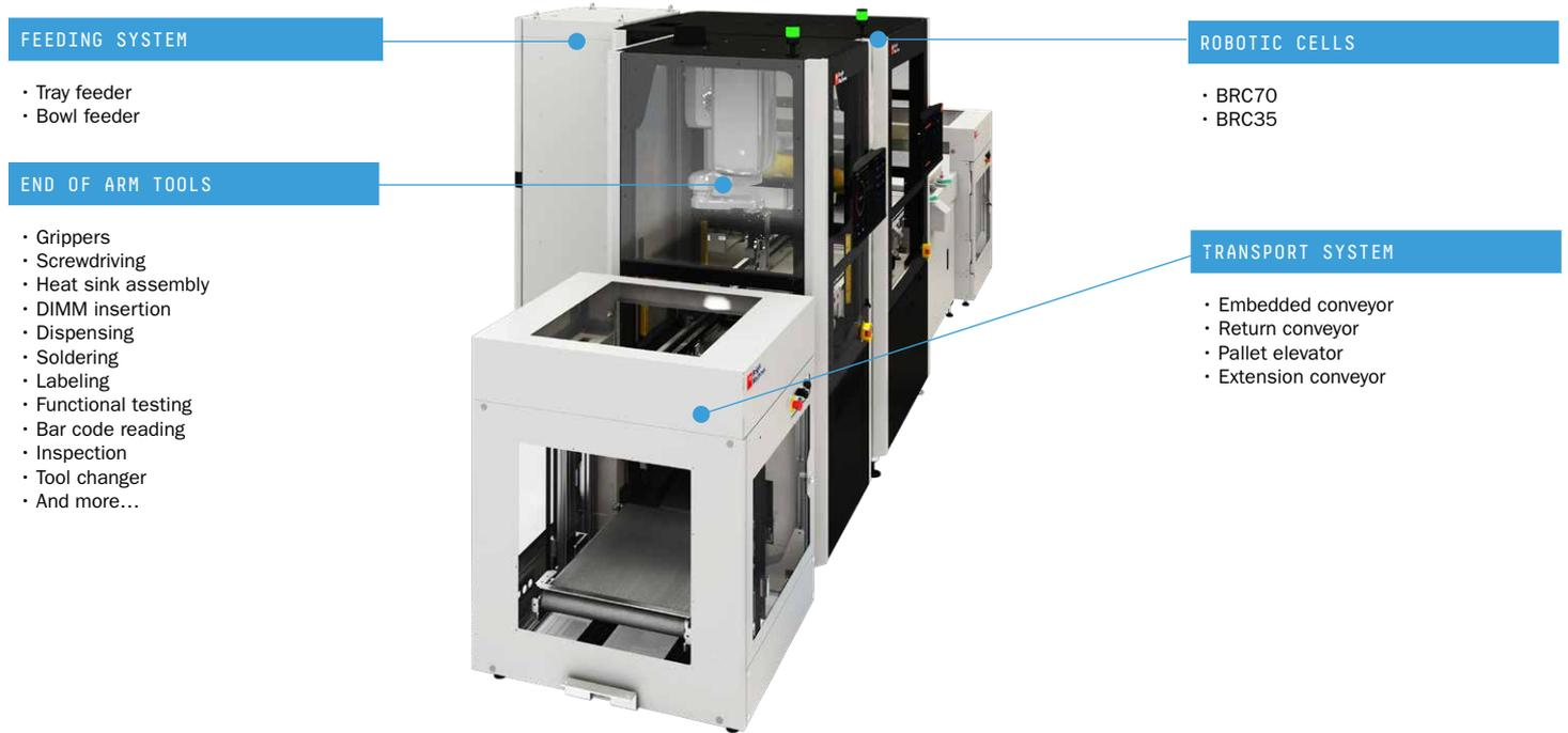
Bright Machines Microfactories are a modular and flexible system. Automation components, whether they are designed by Bright Machines or come from a third party, can be quickly configured to form flexible, scalable assembly lines. And when it comes time to wind down the production on a line, the automation components can be repurposed to build the next product.
