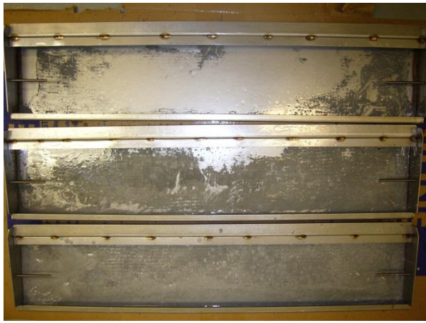
Figure 17: Solder Paste Collected in Sluice Boxes
